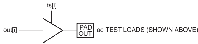
Figure 57. ac Test Loads
